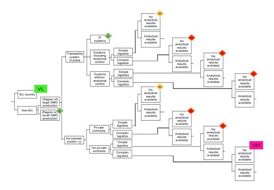
Figure 4 - Decision tree diagram for the assessment of the risk of the presence of UGMs (Žnidaršič et al., 2009).
